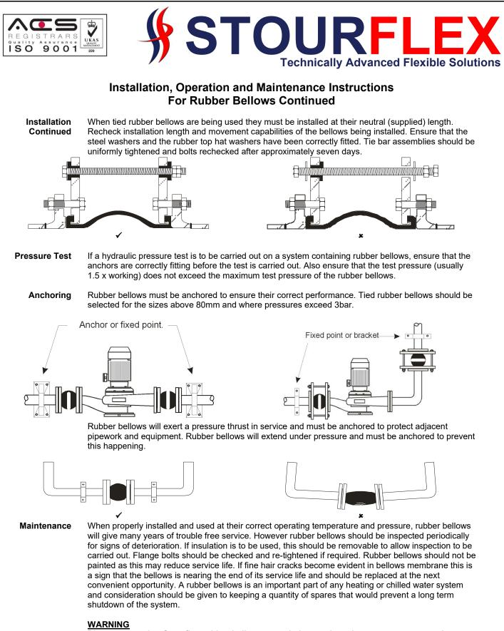
Please note using Stourflex rubber bellows over their stated maximum temperature and or pressure can cause premature ageing of the rubber body and result in burst failure.
