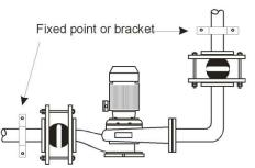
Rubber bellows will exert a pressure thrust in service and must be anchored to protect adjacent pipework and equipment. Rubber bellows will extend under pressure and must be anchored to prevent this happening.
